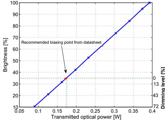
Fig. 4: Brightness versus transmitted optical power.
