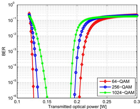
Fig. 7: The average BER versus the transmitted optical power for different modulation orders.
