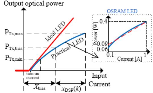
Fig. 2: LED transfer characteristic (optical power vs. forward current).
