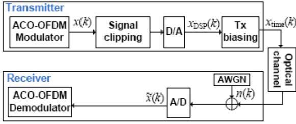
Fig. 1: OWC system based on the ACO-OFDM scheme. Signal clipping is realized in the digital domain.
