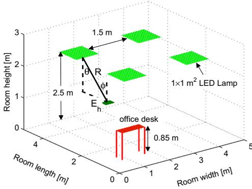
Fig. 3: Model room. Layout of ceiling lighting.
