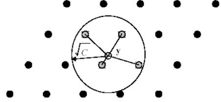
Fig. 8. Schematic of the sphere decoding principle - only the points inside the sphere (grey) are searched
