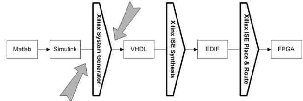
Fig. 3. Hypothetical design flow, the grey arrows show where MIMO concepts can be exploited to improve the final design
