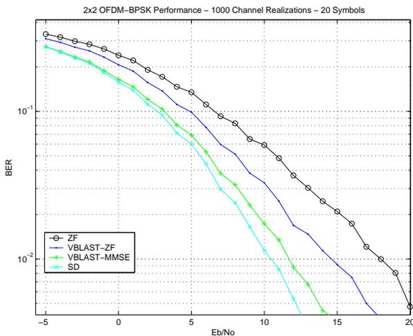
Fig. 10. Bit error ratio performance of MIMO decoding algorithms using OFDM techniques as a function of signal to noise ratio per bit
