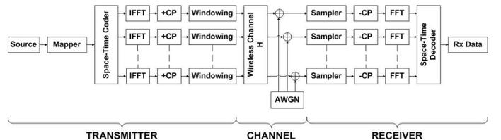
Fig. 7. MIMO-OFDM system block diagram
