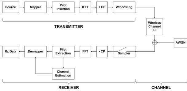
Fig. 4. OFDM system block diagram
