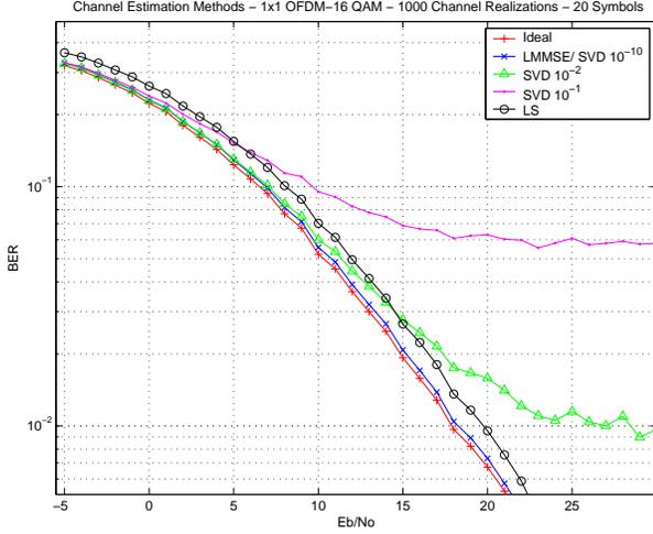
Fig. 6. Bit error ratio performance of OFDM channel estimation methods as a function of signal to noise ratio per bit
