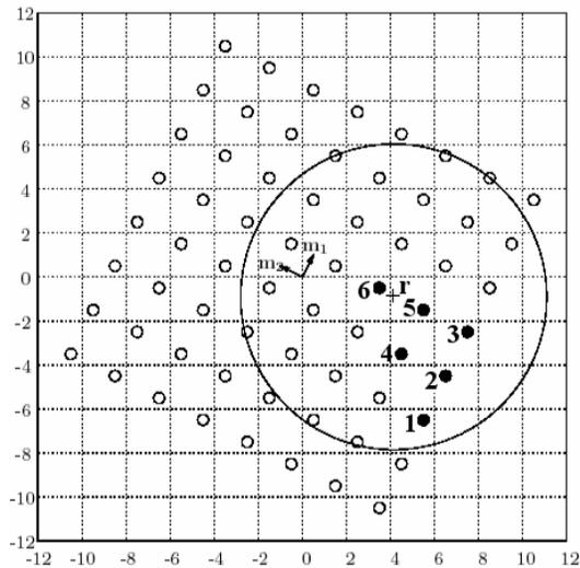
Fig. 9. Operation of the sphere decoding algorithm
