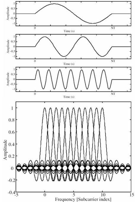
Fig. 1. Subcarriers and frequency spectrum of an OFDM signal
