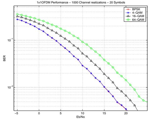
Fig. 5. Bit error ratio performance of an OFDM system under frequency selective fading as a function of signal to noise ratio per bit
