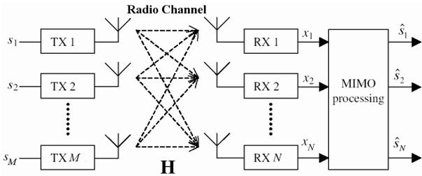
Fig. 2. MIMO communication system with M Tx antennas and N Rx antennas
