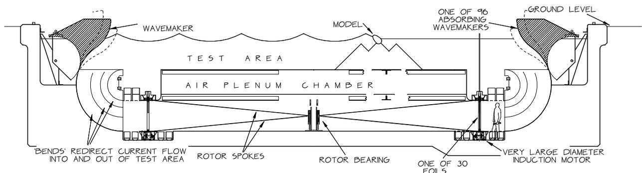
**Figure 18:** Section view of proposed circular combined wave and current tank. The hatched units at either side are elements of the circular array of wavemakers. The moorings of the duck model show the position of the test area floor. At the bottom below the test area is a vertical-axis current generator. Circular 'bends' or guide vanes below the wavemakers direct water from the current generator into and out of the test area. Note the scale of the maintenance engineer at lower right.
